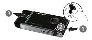
4. Grip the battery at the top end (1) and lift it up and out (2) (as shown).
