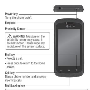
⚠ WARNING: Putting a heavy object on the phone or sitting on it can damage its LCD and touch screen functionality.
