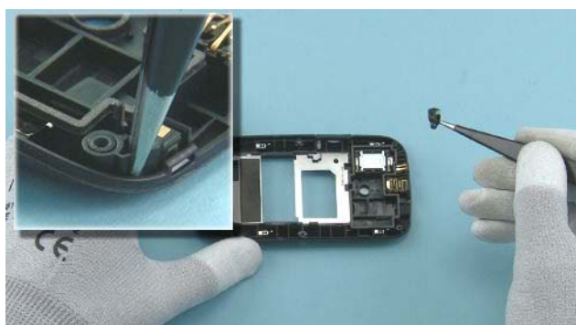
33) Remove the BT/WLAN ANTENNA with tweezers.
