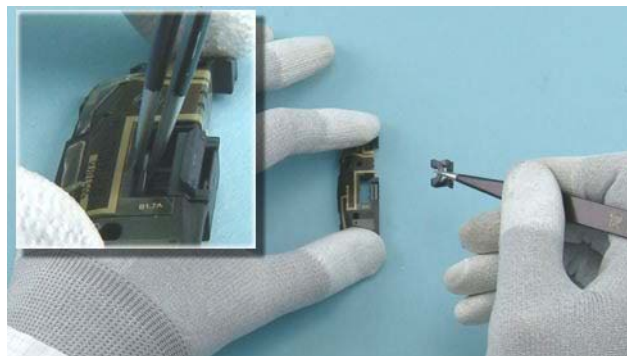
32) Remove the RELEASE BUTTON with tweezers.
