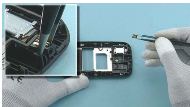
35) Remove the DC JACK with tweezers.
