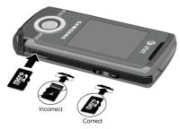
Push the microSD<sup>™</sup> card into the slot until it clicks into place. Warning!: Make sure the printed circuit side of the microSD<sup>™</sup> card is facing down when inserted.
