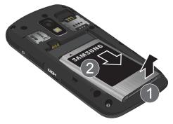
**3.** Lift the battery up and out of the phone (2).
