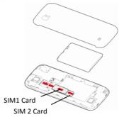
Finally insert the battery and replace the rear cover of the mobile phone.
