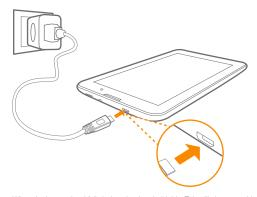
When the battery level falls below the threshold, IdeaTab will alert you with a tone and the battery status icon will change into . We recommend you plug the AC power adapter into your IdeaTab in the direction of the orange arrow as shown above figure.
