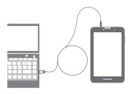
You can connect IdeaTab to the PC's USB port with the cable provided for battery charging or data transferring with the PC.
