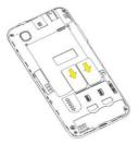
Insert the memory card into the metal slot with the metal contacts facing down until it clicks to the right position.
