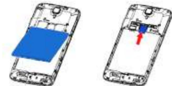
3. Finally place back the battery and rear cover.
