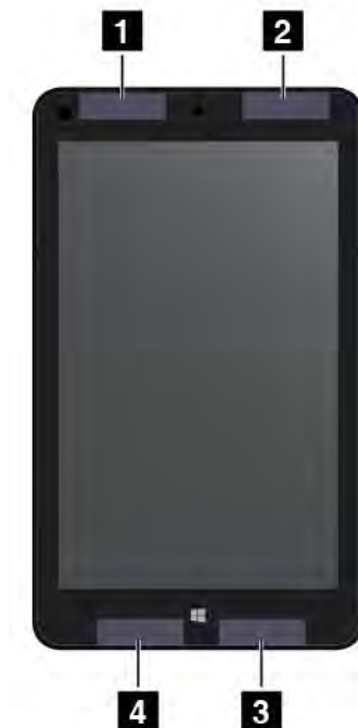
Figure 5. Location of the UltraConnect wireless antennas
