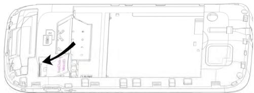
4) With the metallic contacts of the battery facing the metallic contacts in the battery slot, press the battery down until it locks into place, then fix its back co
