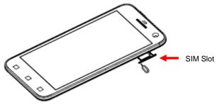
3. Insert the SIM tray of the mobile phone and power on.
