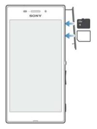
Don't confuse the micro SIM card slot with the memory card slot.
