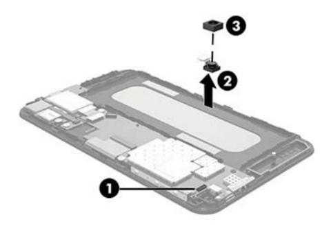
Reverse this procedure to install the rear-facing webcam.
