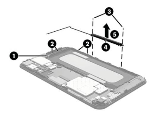
6. Remove the antenna board and cables.
