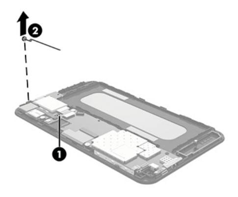
3. Remove the microphone and cable.
