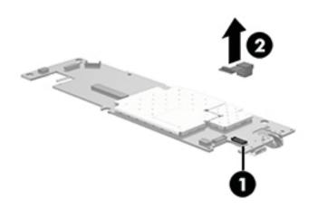
3. Remove the front-facing webcam and cable.
