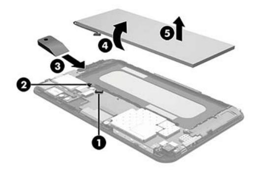
Reverse this procedure to install the battery.
