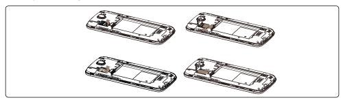
To install SIM card, start by sliding the metal tray up to unlock position, tray will click and release when unlocked. Place the SIM card into the slot with gold contacts facing downward. Once SIM card is placed into slot, close metal tray, then slide tray down, tray will click when locked. Reattach back cover to phone and power phone on. To remove SIM card, slide the metal SIM card tray to unlock position and gently slide the SIM card out from slot.
