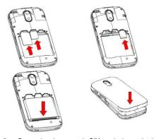
**Attention**: Do not bend or scratch SIM card, do not let it contact with static electricity, dust or water.
