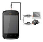
**Tip:** You can also use a compatible USB charger to charge your battery. Use only MAXX approved chargers and cables. Unapproved chargers or cables can cause battery to explode or damage your device. We suggest you charge the battery for 4 hours continuously for the first time.
