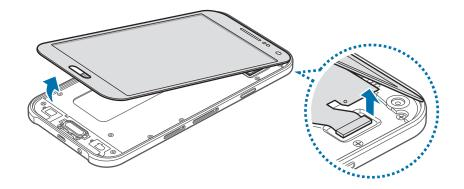
Do not completely separate the front panel from the case before disconnecting the cable. This may result in damage to the device.
