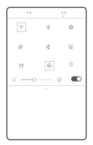
Touch (1) to turn on mobile data. Touch and hold (2) to go to the Wi-Fi settings screen. Turn on Wi-Fi and connect to a Wi-Fi network.
