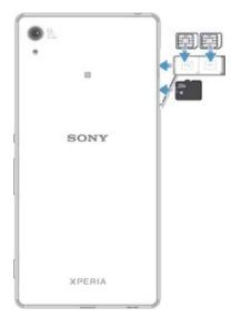
Make sure you place the nano SIM card (or cards) in the nano SIM card holder before inserting the nano SIM card (or cards) into the device. Also, don't confuse the nano SIM card slot with the memory card slot.
