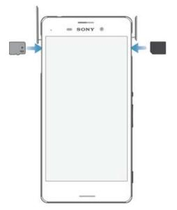
Don't confuse the nano SIM card slot with the memory card slot. Inserting a card in the wrong slot could damage both the card and your device.
