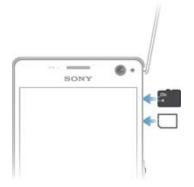
Don't confuse the nano SIM card slot with the memory card slot. Inserting a card in the wrong slot could damage both the card and your device.
