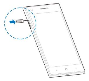
2. Pull out the nano-SIM card tray and place the nano-SIM card in the tray making sure it is properly oriented. Then carefully install the tray back.
