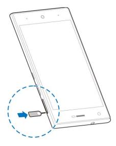
2. Pull out the SD card tray and place the SD card in the tray making sure it is properly oriented. Then carefully install the tray back.
