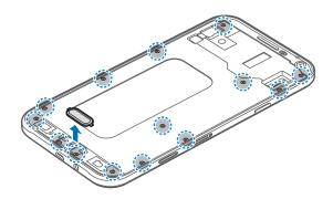
4 Remove the circuit board by lifting it out of the case using an opening tool, then put the case aside and place the circuit board face down on a flat work surface.
