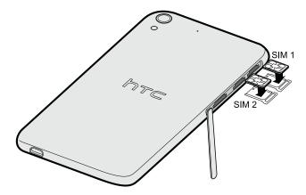
5. When reinserting the trays, make sure they are facing up so that the nano SIM cards don't fall out. Slide the trays all the way into the slots.
