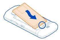
8 To replace the cover, direct the top locking catches toward their slots, and press down until the cover locks into place.
