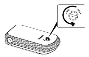
**Note:** The battery cover screw is permanently mounted on the cover and cannot be removed.
