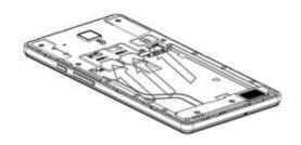
4. Place the battery, align the contacts of the battery with the corresponding connectors in the battery compartment & place the back cover.
