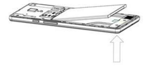
3. Insert the SIM cards and Micro SD card into their respective slots as shown.
