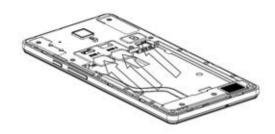
4. Place the battery, align the contacts of the battery with the corresponding connectors in the battery compartment & place the back cover.
