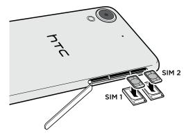
5. When reinserting the trays, make sure they are facing up so that the nano UIM and nano SIM cards don't fall out. Slide the trays all the way into the slots.
