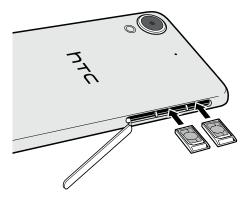
6. Close the slot cover. Press from the bottom to the top of the slot cover to lock it in place.
