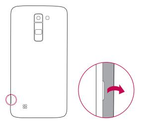
2 Slide the Nano SIM card into the Nano SIM card slot as shown in the figure below. Make sure the gold contact area on the card is facing downward.
