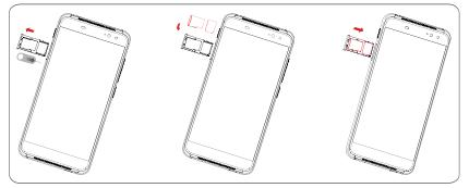
Before you install or remove the SIM card or microSD card, use a pin to press the small cavity until the SIM/microSD slot pops out. Place the SIM card with the chip facing downwards and slide it into its housing. Make sure that it is correctly inserted.
