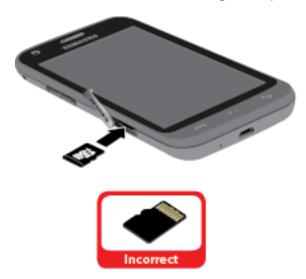
3. Firmly press the card into the slot and make sure that it catches with the push-click insertion.
