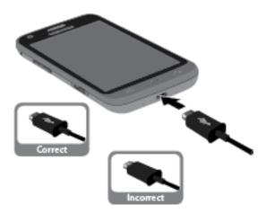
3. Plug the AC adapter into an electrical outlet and charge your battery. Fully charging a battery may take up to three hours.
