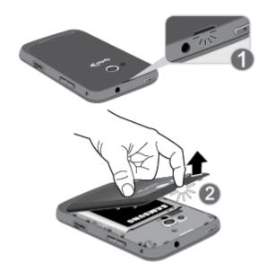
• Insert the battery, contacts end first, and gently press the battery into place.
