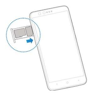
The nano-SIM card, and the microSD card can be installed or removed while the phone is turned on. You need to unmount the microSD (not included) card before removing it.
