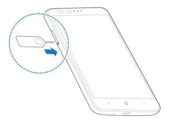
2. Pull out the SIM / SD tray and place the nano-SIM card (right) /microSD card (left) facing down on the tray. Gently slide the tray in until it clicks into place.
