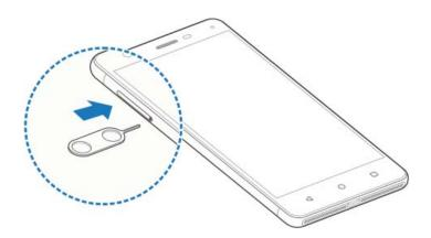
2. Pull out the card tray and place the nano-SIM card (right) /microSDXC card (left) facing down on the tray. Gently slide the card tray in until it clicks into place.
