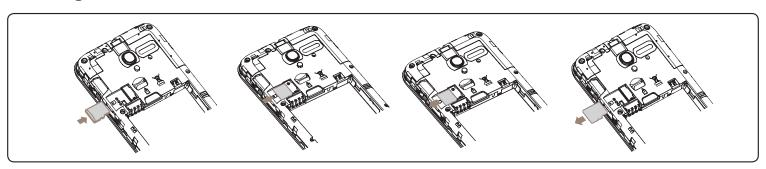
Place the microSD card with the chip facing downwards and slide it into its housing. Make sure that it is correctly inserted. To remove the microSD card, press and slide it out.
