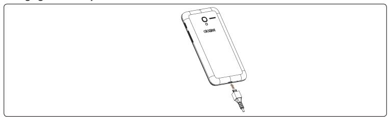
To charge the battery, connect the charger to your phone and mains socket. You can also charge your phone via a USB cable.
