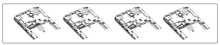
Place the SIM card with the chip facing downwards and slide it into its housing. Make sure that it is correctly inserted. To remove the SIM card, press and slide it out.
