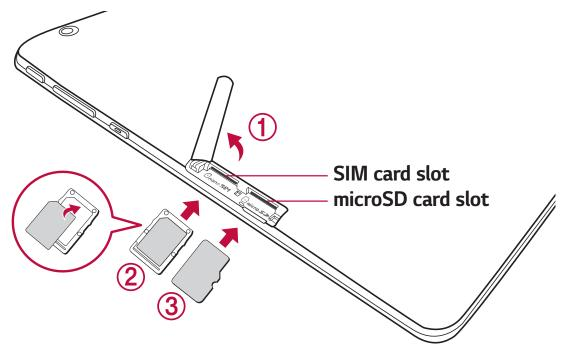
**3** If you want to use a memory card, insert the memory card into the slot. Make sure the gold contact area is facing downward. Slide the microSD card into the slot until it "clicks" into place and then close the slot cover.
