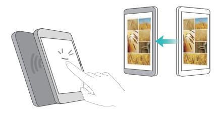
Check that the screen is unlocked on both phones and ensure that NFC is enabled. Enable Android Beam on the other phone (if required).
