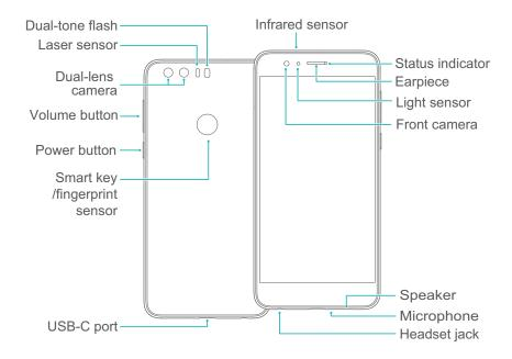
Do not cover the light sensor, as this will affect some of the phone's functions. Ensure that you use a screen protector that has a purpose-built hole for the light sensor.
