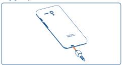
Connect USB Cable provided to your phone and charger, then connect charger to electric outlet. Phone charging icon will display on status bar, confirming battery charging.
