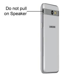
**Warning**: Do not bend or twist the back cover excessively. Using excessive force on the cover during removal or installation of an internal component can cause the material to break.
