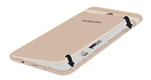
2. Press along the edge of the back cover until you have a secure seal.
