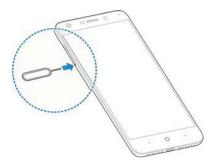
Pull out the card tray and place the nano-SIM card and the microSDXC card on the tray, as shown. Carefully slide the tray back into place.
