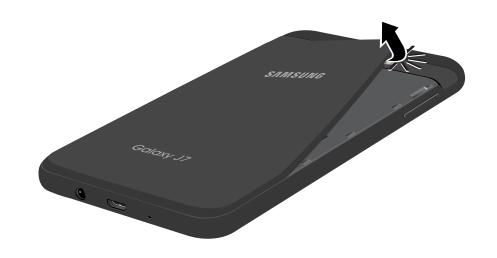
**Caution**: When removing the back cover, use the slot next to the Volume key to gently lift the cover off. Pulling on the Speaker (located next to the Power key) may cause damage.
