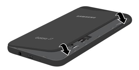
2. Press along the edge of the back cover until you have a secure seal.
