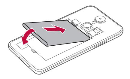
3 To replace the cover onto the device, align the back cover over the battery compartment and press it down until it clicks into place.
