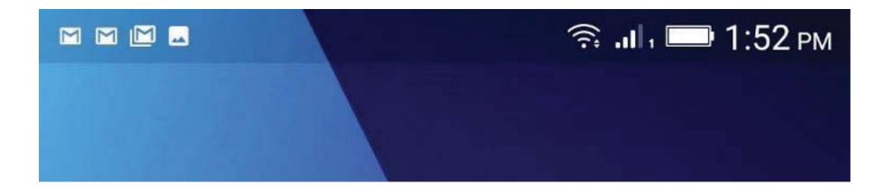
On the notification bar, several icons will appear such as signal bar, time, battery indicator, data indicator, Bluetooth and Wi-Fi. You may slide the notification bar down with your finger to display any pending notifications or actions.
