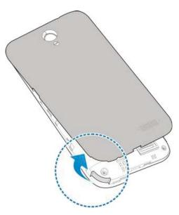
2. Hold the nano-SIM card with the cut corner oriented as shown and slip it into the card holder.
