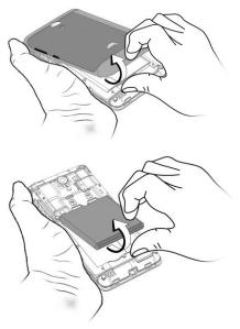
2. Insert the SIM card(s) and memory card as shown:
