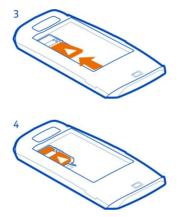
4 Line up the battery contacts, push the battery in (5), then replace the back cover (6).
