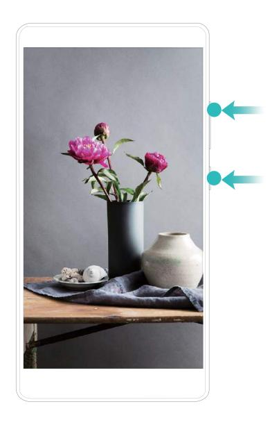
**Use knuckle to start recording**: Knock two of your knuckles to the screen twice in quick succession to start recording. Select **Microphone**, **System**, or **None** from **Sound source** based on your needs. To end the recording, gently and rapidly double-tap the screen with two of your knuckles again.
