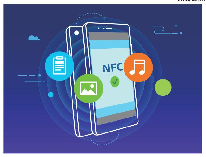
**Use NFC to send data**: Open Settings, then touch Device connection and enable NFC and Huawei Beam. Select the files to be sent and touch Share > Huawei Beam. Keep your Phone unlocked and the screen on. Place the NFC detection areas of both devices close together. Once a connection is established, the transmitting device will play an audio prompt and the sharing screen will minimize. Touch the transmitting device's screen to begin sending files.
