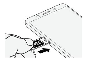
6. Make sure the tray is fully inserted and doesn't protrude from the slot.
