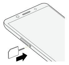
When inserting the eject tool into the tray eject hole to remove the card tray, do not obstruct the tray to avoid damaging the eject mechanism inside the slot.
