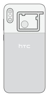
Make sure that the NFC area (shaded part) of HTC U12 life and the other phone's NFC area are close to one another. Experiment by slightly moving the phones until a connection is made.
