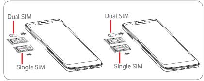
Insert the pin into the hole and pull out the tray. Place the SIM card or microSD card with the chip facing downwards on the tray, and put the tray into its housing. Make sure that it is correctly inserted. To remove the SIM card or microSD card, pull out the tray.
