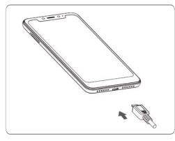
To charge the battery, connect the charger to your phone and mains socket. You can also charge your phone via a USB cable.
