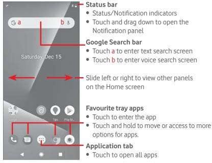
The Home screen extends on either side of the screen to allow more space for adding apps, shortcuts, etc. Slide the Home screen horizontally left and right to get a complete view of the Home screen.
